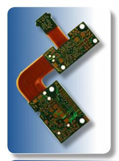
47N is a low-flow epoxy prepreg engineered for bonding multilayer epoxy rigid-flex or attaching heat sinks to multilayer PCBs. An optional reduced lamination temperature protects components already mounted on the PCB.
