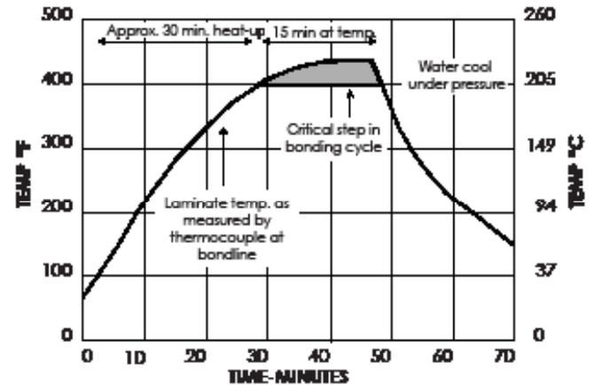
A time-temperature curve as shown on the accompanying chart illustrates a typical press temperature cycle which has produced satisfactory bonding results.
