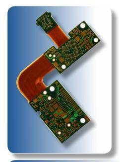
37N is a polyimide low-flow prepreg suitable for bonding multilayer polyimide rigid-flex, attaching heat sinks to polyimide MLBs, or other applications where minimal and uniform resin flow is required.
