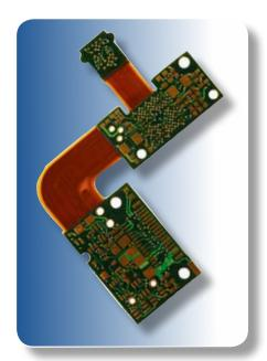
51N-LF is a non-DICY multifunctional epoxy low-flow prepreg system designed to provide high reliability through lead-free solder operations. The high decomposition temperature and high thermal stability of this material is ideal for use in complex rigid-flex fabrication and assembly operations where minimum resin flow is required.
