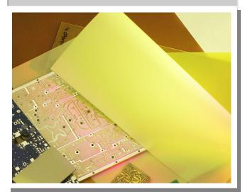
Arlon's AD430 is a woven fiberglass reinforced, ceramic filled, PTFE-based composite material for use as a printed circuit board substrate. It has been developed to provide low loss, low thermal expansion and strong interlaminar and copper bond integrity while maintaining a high degree of affordability.
