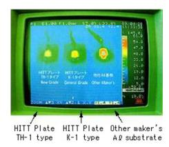
**Comparison of thermal images by thermo-viewer** This photograph shows the thermal mages with a 4A current applied for 10 seconds (Tr: TO-220). It can be seen that the temperature rise of the "DENKA HITT PLATE" is kept very small thanks to its excellent thermal conductivity.
