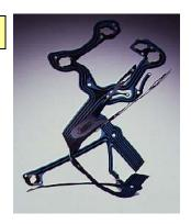
AKAFLEX PENDF HT is available both with different types of **PEN film and thickness grades** as well as with different thickness grades of **adhesive coatings**.
