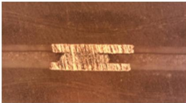
fastRise TM prepreg between subassemblies w/copper paste
